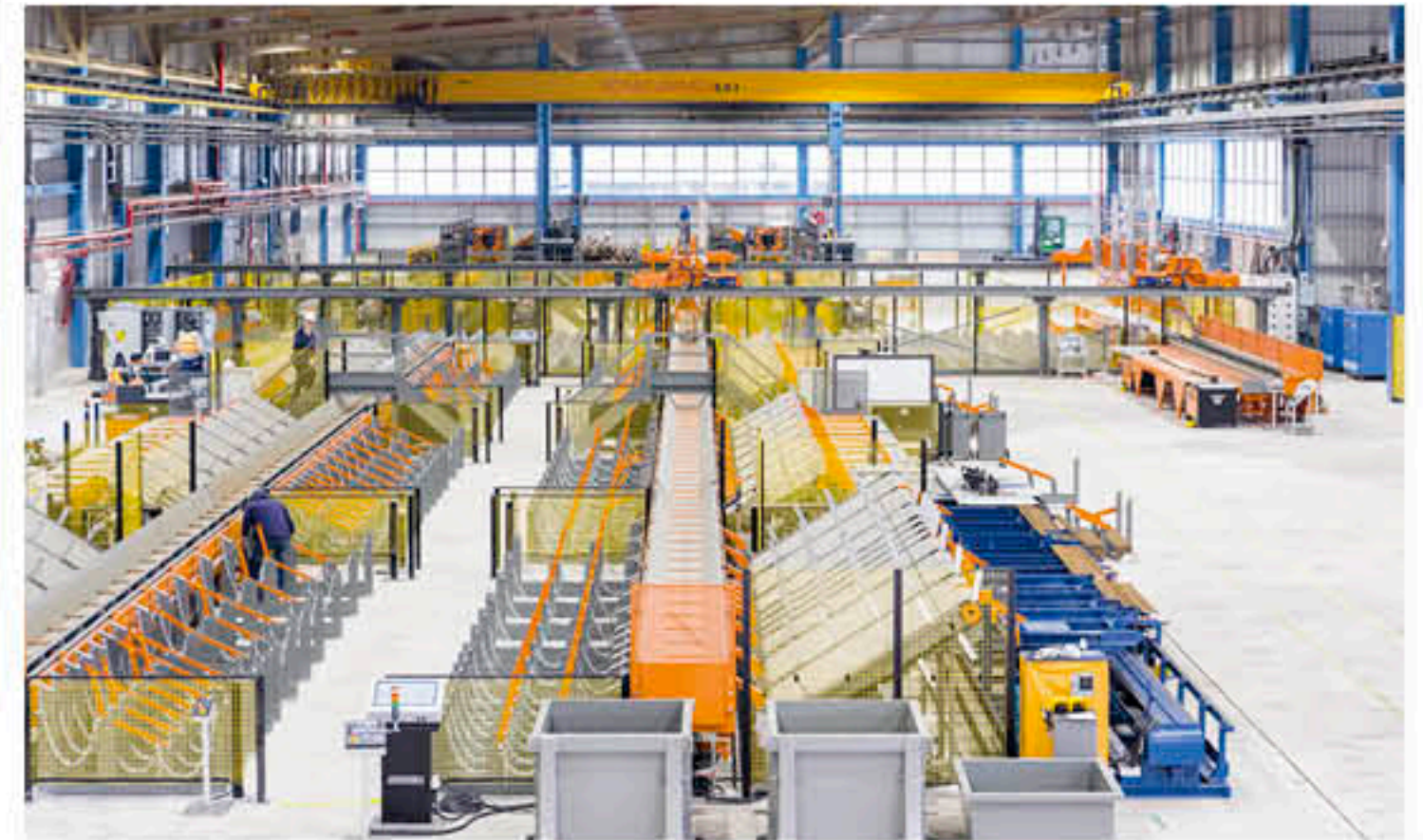
Automated Reinforcement Steel Processing at TVSC
